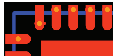
Figure 8. Copper stubs on outer layers.
